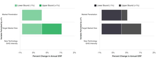
The tornado chart provides a sensitivity analysis. It highlights how the user-defined uncertainty (±1%), when applied to one variable at a time, impacts the final results.
