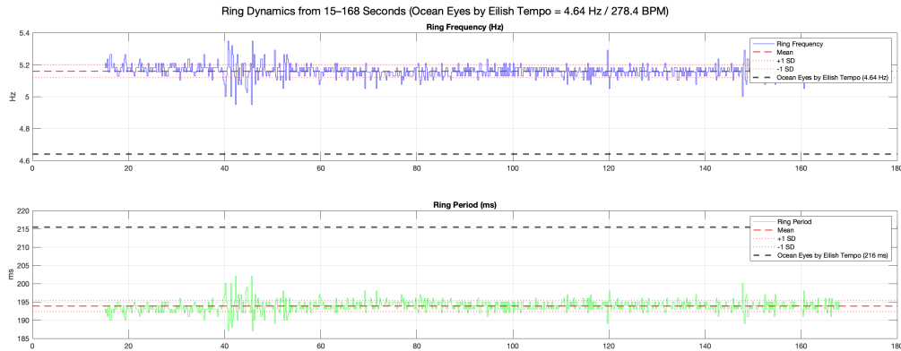
Figure 17: Stimulus: Ocean Eyes by Billie Eilish. Description: PCA ring data was 5.159 \pm 0.040 Hz (period of 193.8 \pm 1.5 ms); song tempo was 4.64 Hz (beat interval of 215.5 ms). Electrodes: 16 total (whole cortex): Fp1, Fp2, C3, C4, Pz, Fz, O1, O2, F7, F8, F3, F4, T3, Cz, P3, P4. Results: https://youtu.be/ezi5fu7uzq0 .
